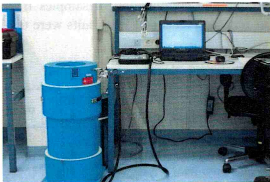
Figure 8: Setup shift register with HLNC detector
